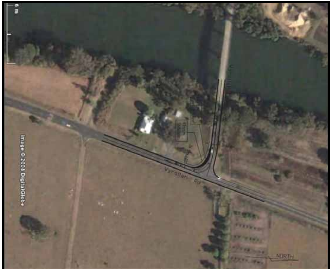
Figure 6.2 Proposed Intersection treatment for Wyrallah Road – Wyrallah Ferry Road (source: RoadNet, 2009)
