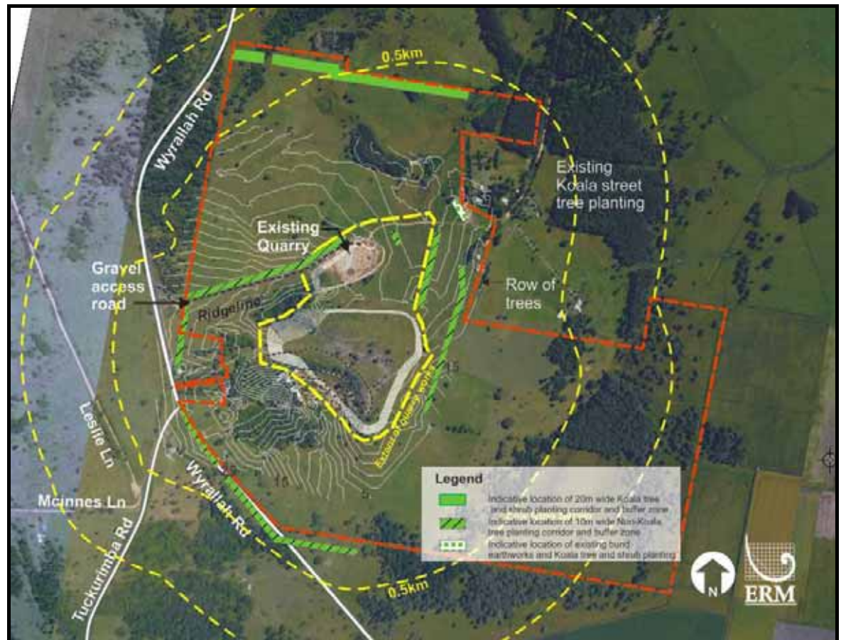
Figure 14.2 Proposed bund construction and tree planting
